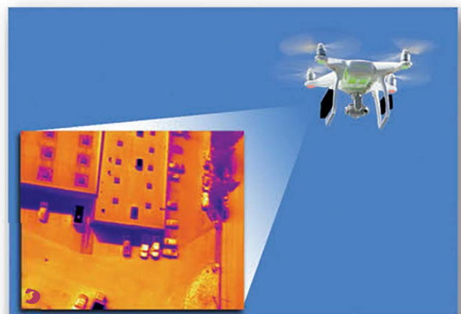
Actual live thermal imaging feed from the PredatIR system in flight
